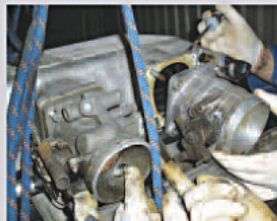
Stripping the throttle bodies off the engine.
